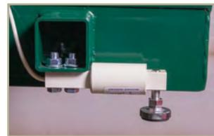
A weigh bar (one of four) mounts under the unit at each corner.
