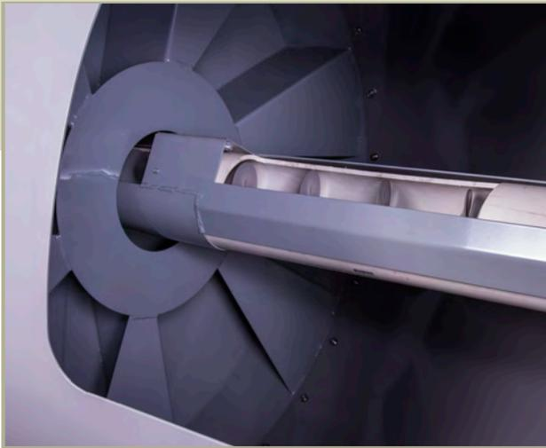
Huge scoops pick up the ration and dump it into an auger that moves the feed forward. With the discharge door closed, the feed drops into the drum and moves to the back for the process to be repeated. A removable cover provides access to the auger.
