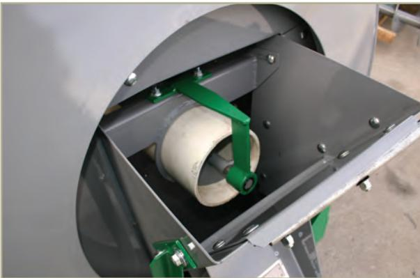
To reduce clatter, heavy wall PVC pipe is used to encase the auger. It's practical, efficient and cost effective.
