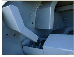
Oversized scoops are secured with stainless steel hardware allowing them to be replaced when required.
