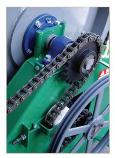
A super strong, quiet synthetic idler for the main drive chain is fully adjustable, while the drum drive utilizes a springloaded idler. All bearings have grease fittings for maintenance.
