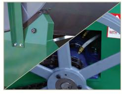
Some bearings have remote grease zerks
